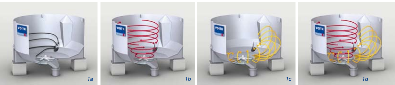
Fig. 1: Flow-pattern in the IntensaPulper IP-R: heavy contaminant removal (black arrows), intensive turbulence (red arrows) and low-level turbulence zone (yellow arrows).
