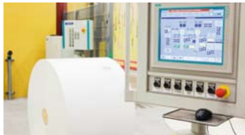
Parent roll transport with fully automated barcode labeling unit.
