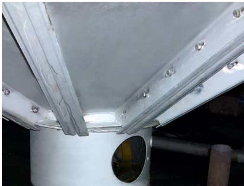
Segmented cone-shaped reactor bottom.
