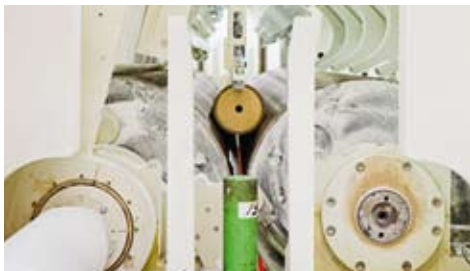
Precise inserting of cores into carrier roll bed.
