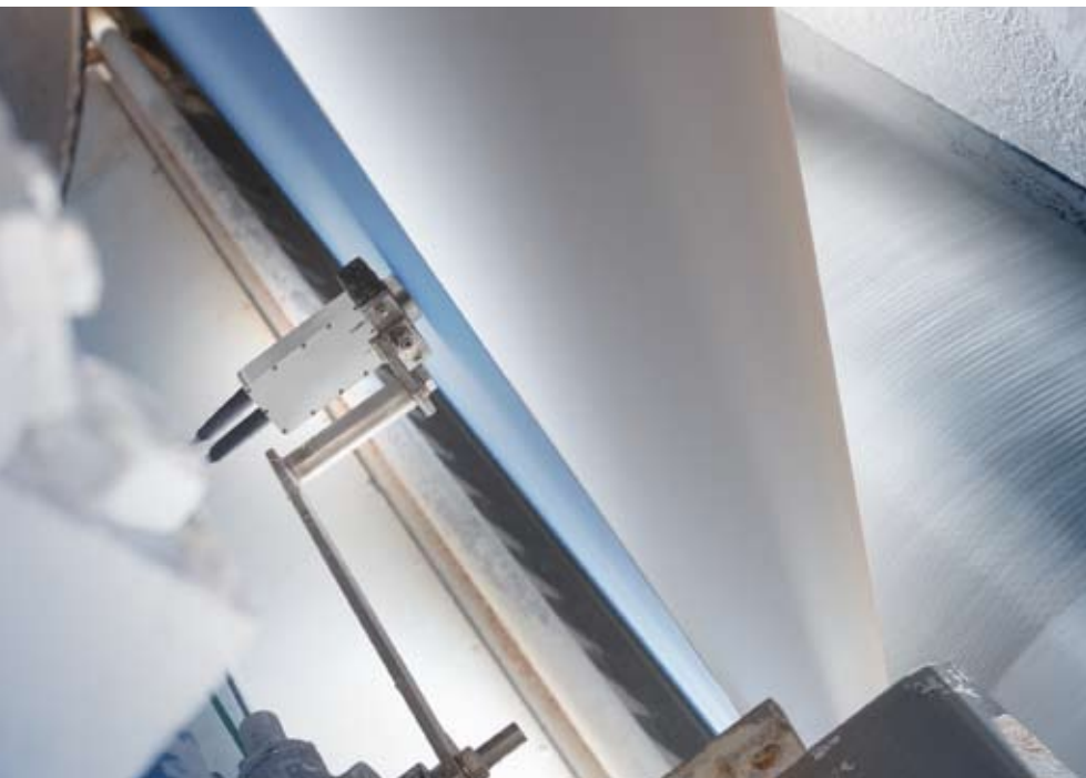
The sensor does not leave any marks on the forming fabric or paper.
