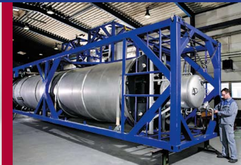
Full-size R2S anaerobic EGSB pilot reactor ready for the first installation
