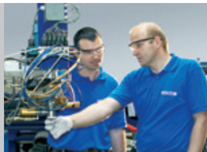
Mixing head of a casting machine for roll covers
