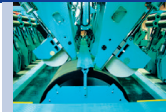
VariTop winding stations operating at 3,000 m/min
