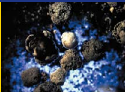
Lime scaling on sludge pellets
