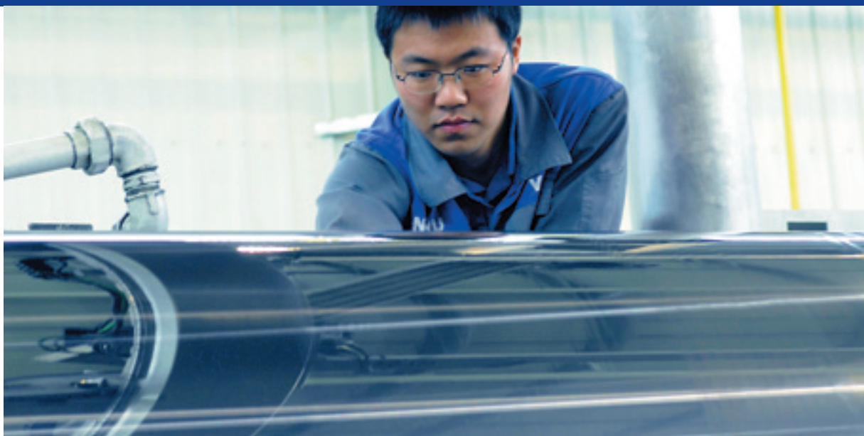
Grinding of a CeraCal Plus roll cover
