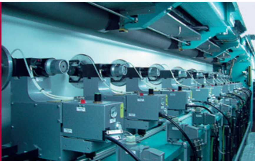
VariTop slitter section (patented)
