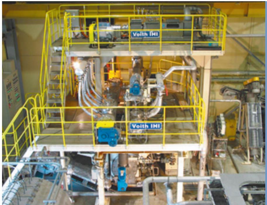
Fig. 2: Trial dispersion system for thickening and dispersion at temperatures up to 125 °C.
