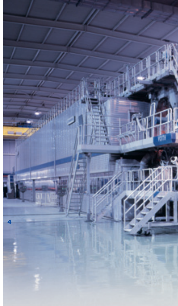
Fig. 4: PM 6 with an annual production capacity of 180,000 t of newsprint.
