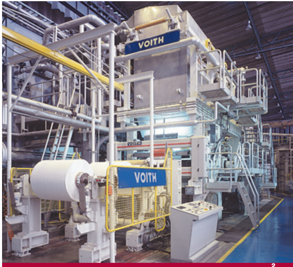
Fig. 2: Tissue-pilot machine at the Process Technology Center at São Paulo, Brazil.
