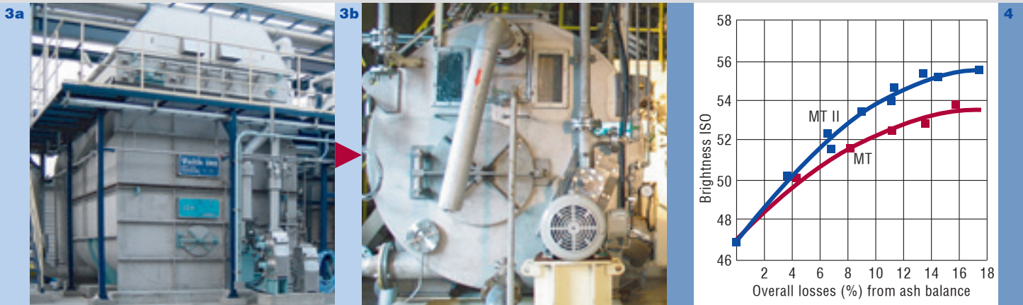
Fig. 4: Overall losses and brightness gain in the primary stage of a pre-flotation system (70% ONP, 30% OMG, 15% ash, soap as collecting agent).
