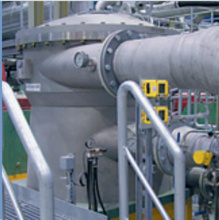
Fig. 8: Part of the Voith stock preparation system with Thune screw press (center).
