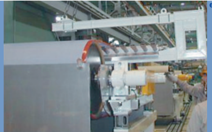
Fig. 6: The maintenance-friendly headbox of the new Compact Washer.
