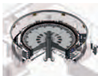
Generator rotor with shaft-coupled, which is lifted down inside stator
