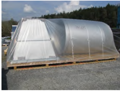
Figure: Clean, rain and dust-proof covering with PE foil
